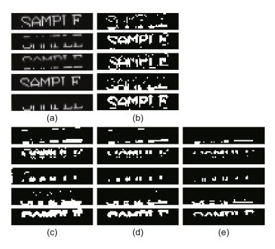
Fig. 5. The observed low-resolution images (a), the weights of pixels given by our proposed method based on the spatio-temporal analysis and automatic thresholding (b), and those given by the existing method based on the median and manual thresholding: (c) t = 0.05, (d) t = 0.1, and (e) t = 0.2. White pixels stand for outliers with w = 0.
