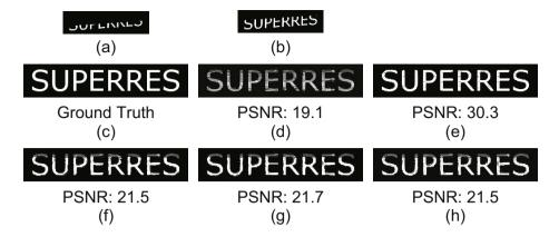
Fig. 9. Super-resolution reconstruction (synthetic): an input image (a), the median image (b), the ground truth of a high-resolution image (c), the conventional method without outlier removal (d), our proposed method (e), and the median-based method with (f) t = 0.05, (g) t = 0.1, and (h) t = 0.2.
