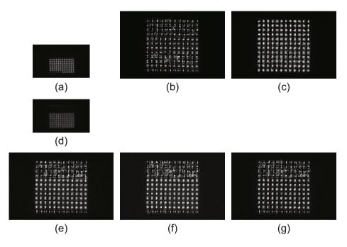
Fig. 8. Super-resolution reconstruction (square): an input image (a), the conventional method without outlier removal (b), our proposed method (c), the median image (d), and the median-based method with (e) t = 0.05, (f) t = 0.1, and (g) t = 0.2.
