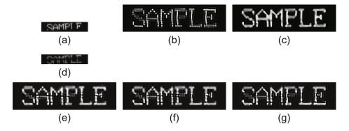
**Fig. 6.** Super-resolution reconstruction (SAMPLE): an input image (a), the conventional method without outlier removal (b), our proposed method (c), the median image (d), and the median-based method with (e) t = 0.05, (f) t = 0.1, and (g) t = 0.2.
