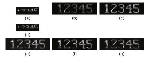
Fig. 7. Super-resolution reconstruction (12345): an input image (a), the conventional method without outlier removal (b), our proposed method (c), the median image (d), and the median-based method with (e) t = 0.05, (f) t = 0.1, and (g) t = 0.2.
