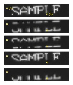
**Fig. 4.** Classification of true background and false background based on temporal analysis: we consider a dark pixel in a certain frame as (a) true background if all of the corresponding pixels in the different frames are also dark or (b) false background if at least one of the corresponding pixel in the different frame is bright.
