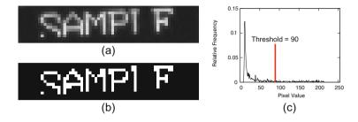
**Fig. 3.** True foreground detection based on spatial analysis: an observed image (a) is binarized by thresholding (b). The threshold is automatically determined from the histogram of pixel values (c) in the observed image on the basis of discriminant criterion. White pixels stand for true foreground.
